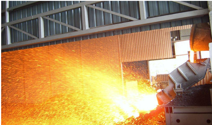
Slag Atomizing Technology is a new process that makes PS Ball blasting media.
