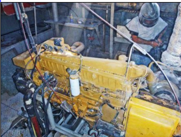
A marine engine being cleaned of corrosion by an Ecoblast® operator.
