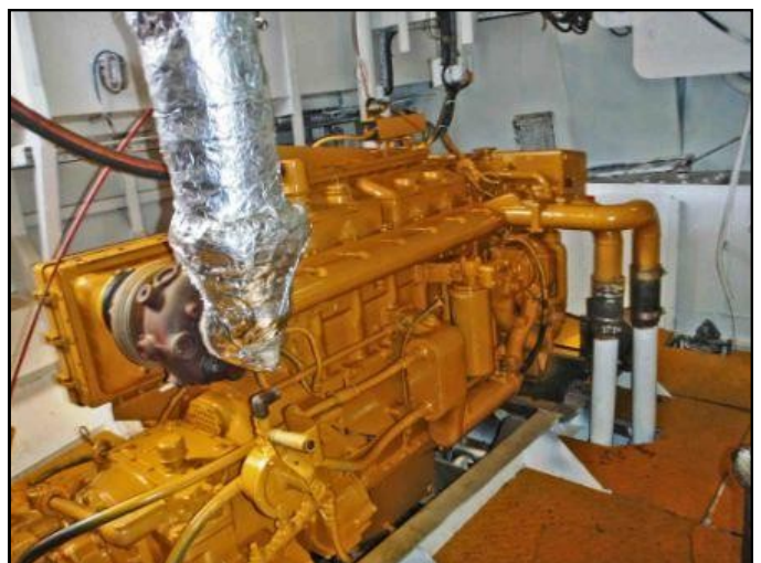
Marine diesel engine after Sodablast treatment.
