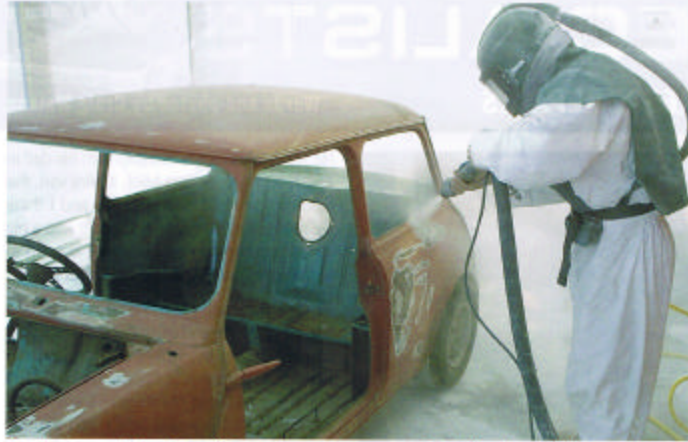
Starting to get the paint off. The soda comes out at 120psi, but doesn't do any damage.
